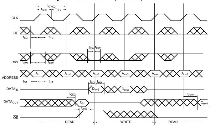
Figure 12. Read with Address Counter Advance<sup>[41]</sup>
